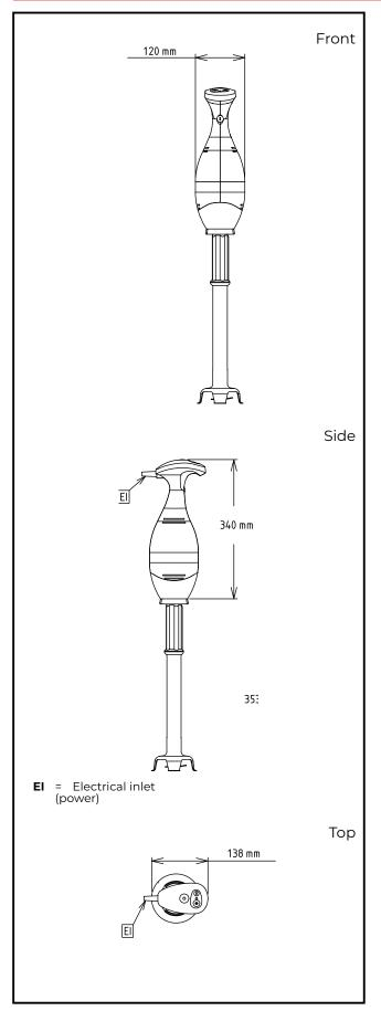
Electric Supply voltage: 220-240 V/1 ph/50/60 Hz **Electrical power max.:** 0.55 kW 0.55 kW **Total Watts:** Key Information: External dimensions, Width: 138 mm External dimensions, 120 mm Depth: External dimensions, 340 mm Height: **Shipping weight:** 3.57 kg
